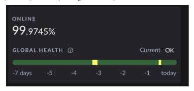
The entity Health is computed based on active alerts. In order to know the health of an entity as it was in the past, we would need to collect alerts that were active for this specific past time. As soon as the Platform or Storage Admin identifies a time at which the entity was degraded, he can access the detailed list of sub alerts impacting this entity.
