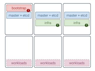
Machines dedicated to the control plane do not require many resources (see *the sizing notes below*), and can safely run as virtual machines. Running workloads on dedicated machines makes them simpler to size, as MetalK8s impact will be negligible.
